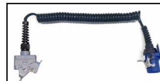
One coiled trailer cable with Harting interface (10 pole Orlaco female) on trailer end and a standard 7-pole connector at the truck end delivered in the cab (FPC11104AJ, AK, DE, DF & DG)
