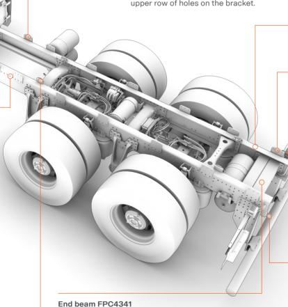
Vehicles that do not have drawbeam, tow beam or any other type of crossmember mounted at the rear of the frame must be fitted with an end beam.
